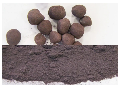
1 kg Ore in DM 200 in 6 min, < 400 \mu\text{m} . Image Credit: RETSCH
