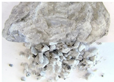
10 kg Diorite in BB 300 with a gap of 1 mm in 1.5 min. Image Credit: RETSCH
