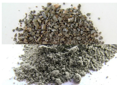
10 g Ore in MM 400 in 2 min, < 100 \mu m. Image Credit: RETSCH
