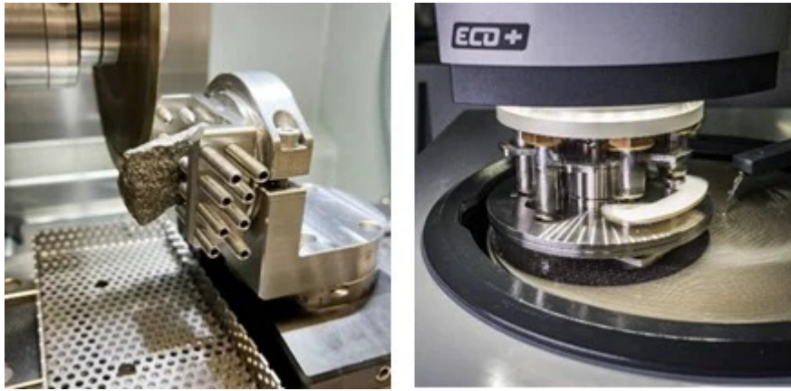
End-to-end geology preparation workflow: Cutting, mounting/impregnation, grinding & polishing, and thin section preparation. Image Credit: QATM
