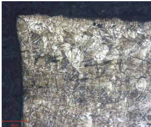
Fig. 7: Etched specimen using "V2A Beize" (for 45 s). Edge section. The microstructure is clearly discernible.
