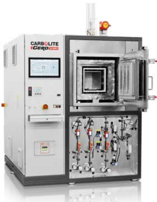
Fig. 6: HTK Metallic Chamber Furnace for debinding and sintering of injection moulded and additive manufactured parts up to 1450^\circ\text{C} .
